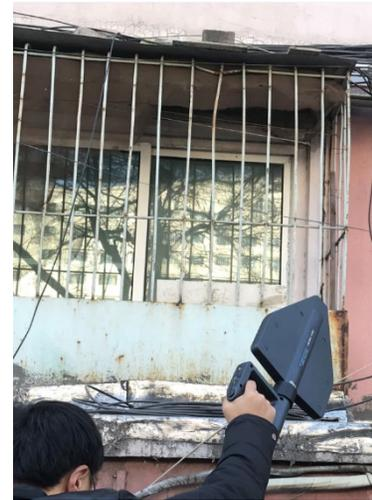
Figure 10 - Localizing PIM with a portable receiver and directional antenna
