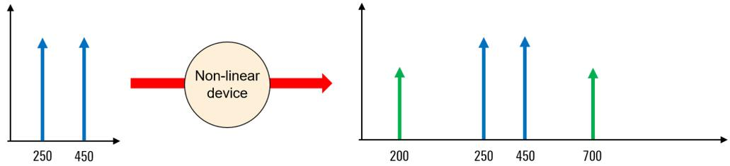
Figure 2 - Intermodulation products
