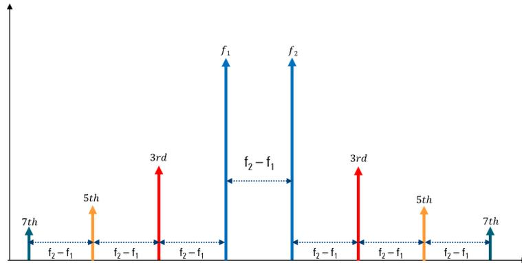
Figure 4 - Spacing of higher order intermodulation products
