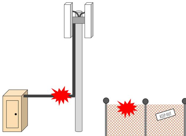
Figure 7 - Internal vs. external PIM sources
