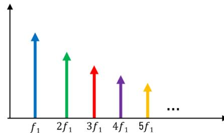
Figure 1 - Harmonics and amplitude
