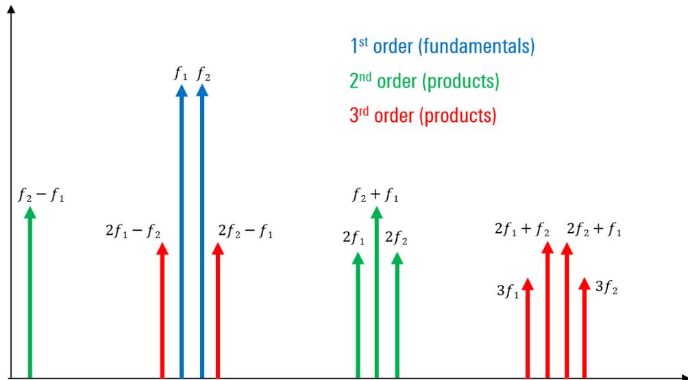
Figure 3 - Fundamentals, harmonics, and products
