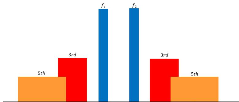
Figure 5 - Width of fundamentals and intermodulation products
