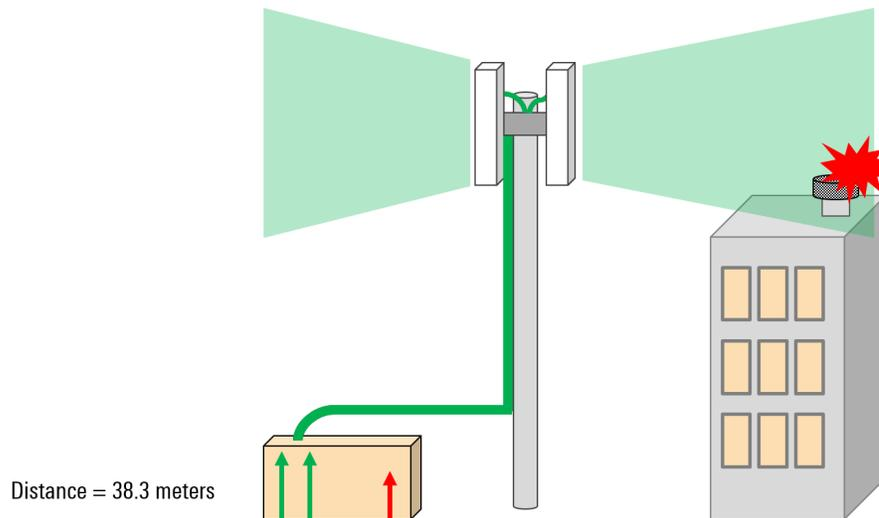
Figure 9 - Distance to PIM (external source)
