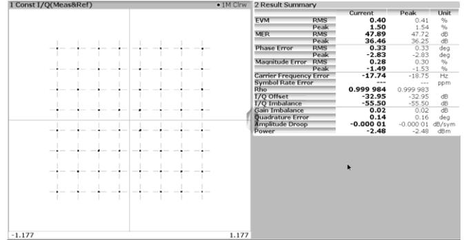
Fig. 4. The measured and demodulated, outphased 64-QAM signal.
