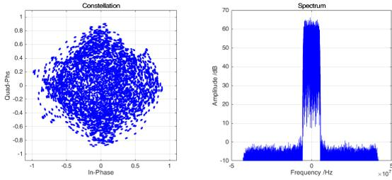
Fig. 2. Reference signal (64-QAM) constellation and spectrum, as used in this paper, shown after transmit filtering.
