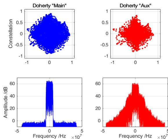
Fig. 7. The decomposed Doherty “Main” and “Auxiliary” signals.
