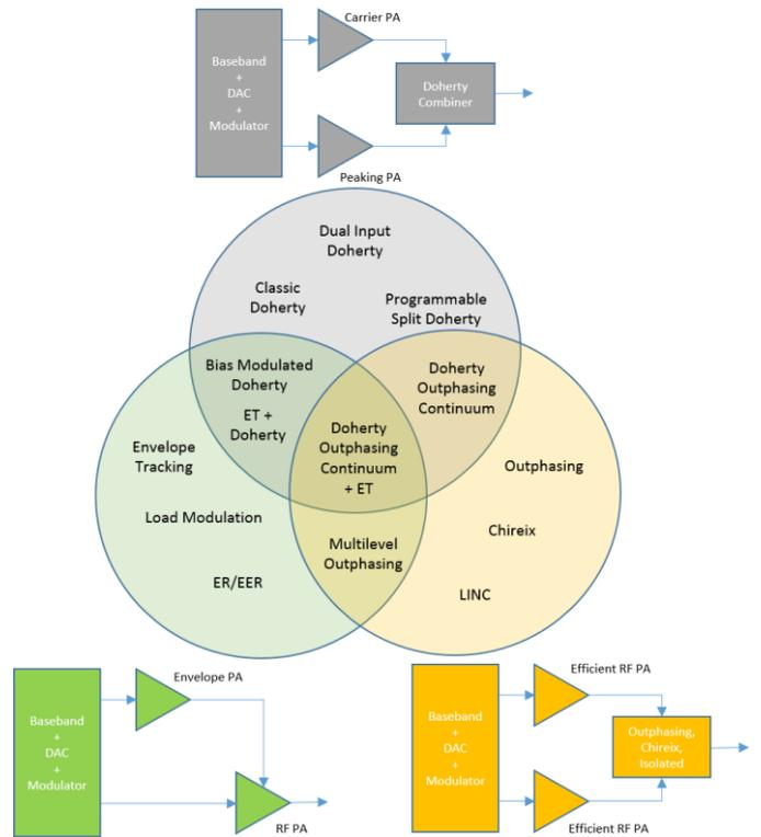
Fig. 1. Predictive, post-correction architectures, based on Outphasing [4], Doherty [1] and Envelope Restoration (ER) [2], adapted from [10].
