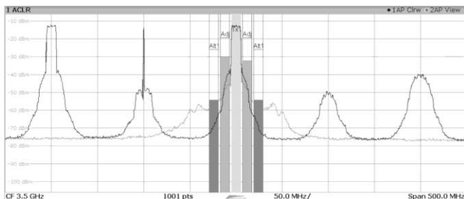
Fig. 6. Output spectrum of the ER generated signal (LO = PM, IF = AM), superimposed with the conventional IF (LO = CW, IF = QAM).
