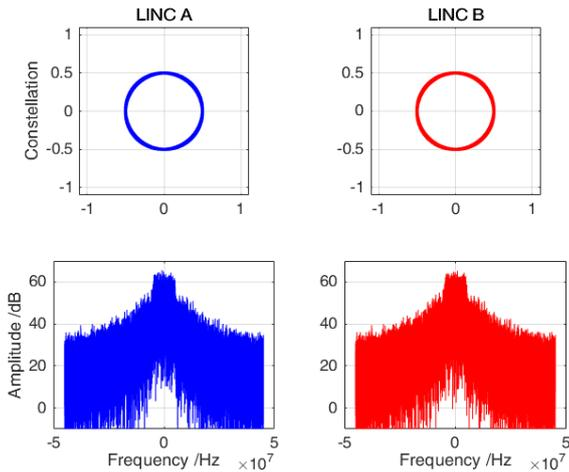
Fig. 3. The two decomposed Outphasing-LINC signals, shown in constellation and magnitude spectrum form.
