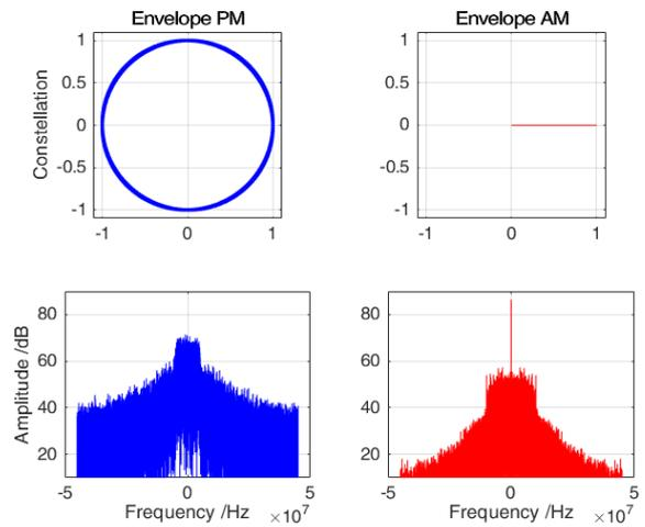
Fig. 5. The two decomposed ER signals, shown in constellation and magnitude spectrum form.
